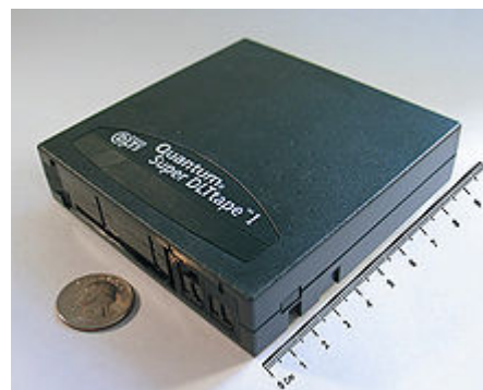
160 GB SDLT tape cartridge, an example of off-line storage. When used within a robotic tape library, it is classified as tertiary storage instead.
