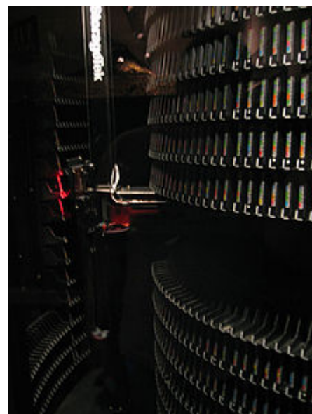
A large tape library, with tape cartridges placed on shelves in the front, and a robotic arm moving in the back. Visible height of the library is about 180 cm.
