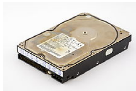
15 GiB PATA hard disk drive (HDD) from 1999; when connected to a computer it serves as secondary storage.
