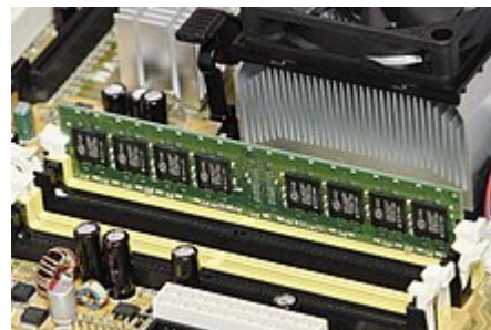
1 GiB of SDRAM mounted in a personal computer. An example of primary storage.
