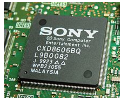
MIPS R3000A-compatible (R3051) 32bit a 33,8688 MHz della playStation
