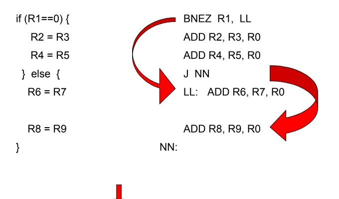
CMOVZ R2, R3, R1(conditional move: if R1=0 then R2=R3)CMOVZ R4, R5, R1(conditional move: if R1=0 then R4=R5)CMOVN R6, R7, R1(conditional move: if R1 $\neq$ 0 then R6=R7)CMOVN R8, R9, R1(conditional move: if R1 $\neq$ 0 then R8=R9)
